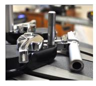
The string clamp portion is very robust and is of the "fit over" design. This allows for a fairly small diameter which can allow a closer fit between the two clamp bases.
