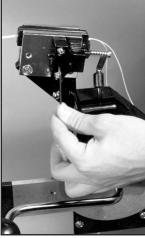
Loosen the locking screw that is located on the side of the black housing block.
