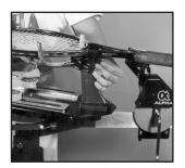
When the crosses are completed, tie off and trim the excess string. To release the racquet, release the pressure on the mounting arms by loosening the adjustment knobs counter clockwise.
