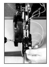
pound increments. For example, to set the tension at 62 lbs, turn the knob so that the marker matches the 60 lbs hash mark on the scale. The 0 hash mark should be lined up with the platform's hash mark. Next, turn the collar two one-pound increments. The 2 lb hash mark should now be aligned with the platform's hash mark. Your tension setting is now 62 lbs. NOTE: When the machine is not in use, release the tension on the spring by setting the tension back down to 9 lbs.
