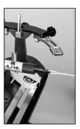
Read the tension on the calibrator to determine if the tension is correct or not.
