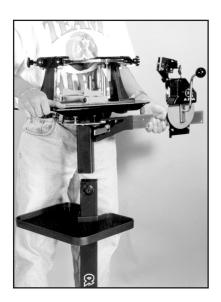
Insert the mounting unit/ tension arm shaft into the pole. For proper balance, make sure the tension arm is extending over the long toe of the base.
