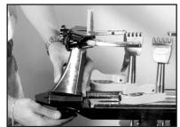
To accommodate the length of each racquet, adjust the mounting arm post by loosening the mounting post adjustment knob. Once the correct
