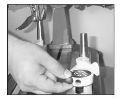
Turn the swivel base so that the outer port is aligned with the inner port. Take the 3mm allen key and insert into the internal adjustment screw. Turn clockwise to increase tension. The ideal locking position for
