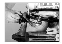
Make adjustments by turning the fine adjustment knobs. The fit should be snug.
