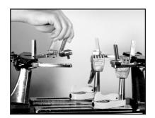
Insert the angle frame supports into the appropriate slots located on the end of the mounting arms. The two slots are designed to accommodate most racquets.
