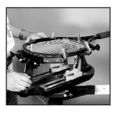
are using a one-piece string job you do not need to make a starting knot. When pulling the crossses across the mains make sure to slide the crosses up and down the mains to disburse the friction in order to prevent 'notching'.
