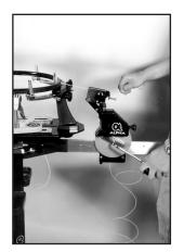
Take the 1st right main and load the string in the jaws of the linear gripper. After loading the string, pull it at an angle to create resistance and to prevent the string from slipping. Grab the handle and rotate the tension head away from the racquet. Keep rotating until the
