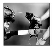
Once the string has been clamped, release the string from the tension head by holding the handle with the left
