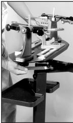
Turn the mounting table so that both mounting posts are perpendicular to the tension head. Lock the mounting table in place by pulling the locking lever out.
