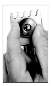
To tighten, turn the dial clockwise. To loosen, turn the dial counter-clockwise. NOTE: Before stringing a racquet, the tension on the string clamp has to be adjusted in accordance with the type of string gauge being used. If the string is of a thin gauge (16L, 17, 18) then the string clamp may need to be tightened. If the string gauge is thick (15, 15L, 16) then the string clamp may need to be loosened.
