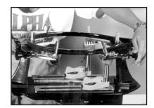
Turn the mounting arm adjustment knobs so that the angled frame supports fit up against the frame. The fit should be snug, but use caution. NOTE: Over-tightening can cause premature stress on the frame.
