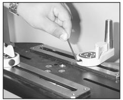
the lever should be down the center of the swivel base.
