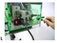
J. Choose the proper electric voltage setting based on the out put in your world region. (110V/220V)
